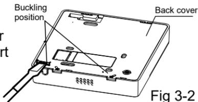
**NOTE:** Do not pry up and down, you can only rotate the screwdriver.
