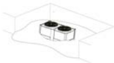
(e) Equipment covered with snow
