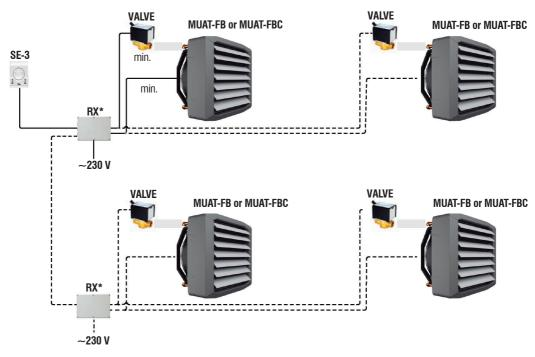
\*Note: Max. 3 RX concentrators to an SE-3 control (or similar); Max. 12 units MUAT-10/20/30-FB; Max. 6 units MUAT-25/40/55 and MUAT-10-FBC; max. 1 unit, MUAT-75/100-FB and MUAT-20-FBC; to each RX concentrator.
