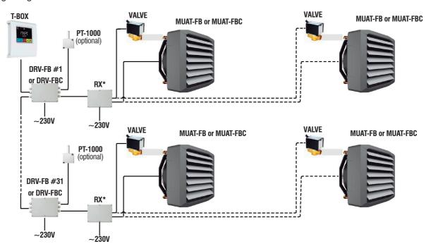
\*Note: Max. 3 RX concentrators to an SE-3 control (or similar); Max. 12 units MUAT-10/20/30-FB; Max. 6 units MUAT-25/40/55 and MUAT-10-FBC; max. 1 unit, MUAT-75/100-FB and MUAT-20-FBC; to each RX concentrator.
