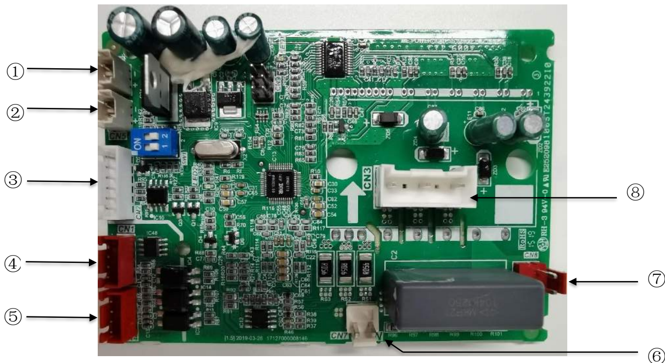
Figure 5-5.1: DC fan drive board ports 1
