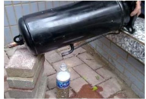
Figure 6-2.8: Draining oil from a compressor
