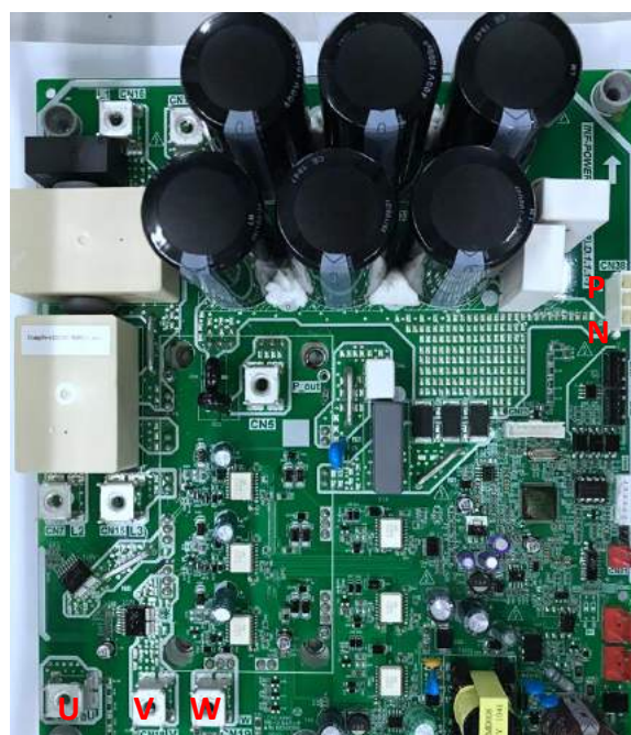
Figure 6-2.1: Compressor drive module terminals
