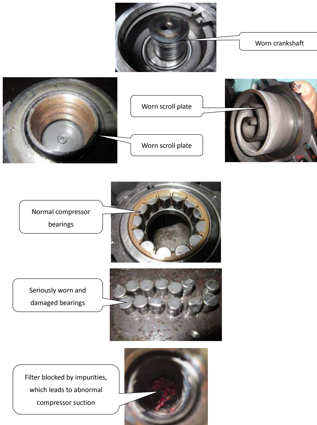
Figure 6-2.11: Effects of spoiled compressor oil
