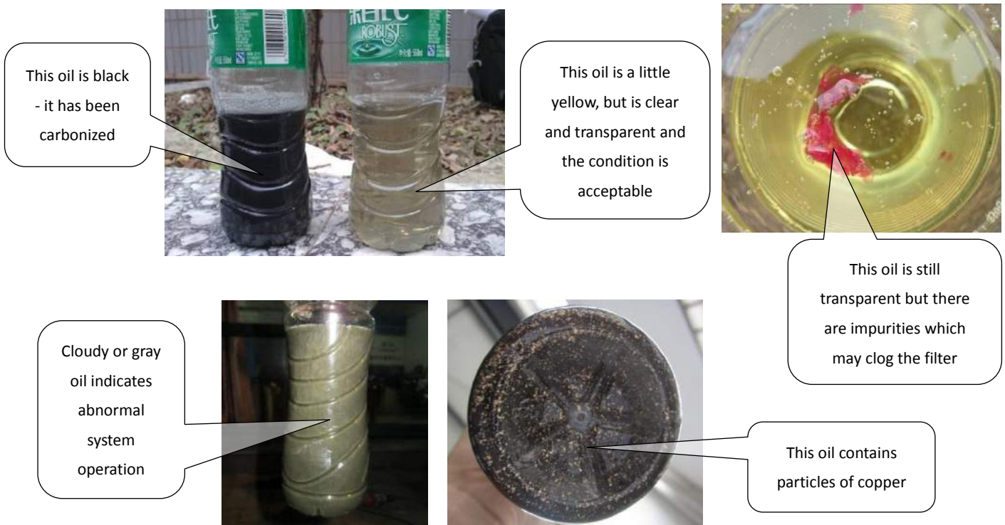
Figure 6-2.10: Inspecting compressor oil
