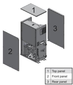
To open the electric control box and operate the interior of the electric control box, open the electric control box cover plate. To open the electric control box, you can open the front panel without needing to open the top or rear panel.
