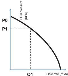
Assume that the performance curve of the selected water pump is as shown in the black figure. When total water resistance in the water system is P1, the flow rate is Q1. When Q1 is within the allowed range of the hydro module, the water pump is suitable. When Q1 is greater than 2.9 m³/h, water pump capacity can be decreased. When Q2 is less than 1.2 m³/h, the water pump capacity should be increased.
