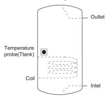
If the tank volume is greater than 240L, the temperature probe (Ttank) should be installed at a position higher than half of the tank's height.
