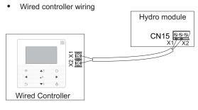
Wires X1 and X2 do not have polarity requirements
