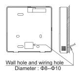
Avoid the water enter into the wired remote controller, use trap and putty to seal the connectors of wires during wiring installation.
