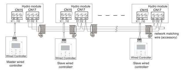
The hydro module can connect the KNX gateway via D1\D2\E so that the third-party wired controller can control the hydro module. In this case, X1 and X2 can be used for check query by connecting or without connecting the wired controller, but cannot be used for control. Equipment which connects to the KNX gateway need to meet SELV regulation.
