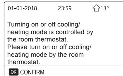
② The room thermostat is SET DOUBLE ZONE(see "ROOM THERMOSTAT SETTING" in "Installation and owner's manual (M-thermal split indoor unit)"). The room thermostat for fan coil is turned off, the room thermostat for the floor heating is turned on, and the unit is running, but the display is OFF. The following page is displayed:
