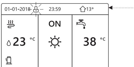
The interface will be locked if there is no handling for a long time (about 120 seconds; it can be set by the interface, see "6.7 SERVICE INFORMATION".)
