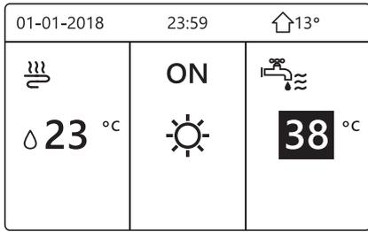
2) When the cursor is on the temperature of DHW mode. Press "ON/OFF" key to turn on/off the DHW mode.
