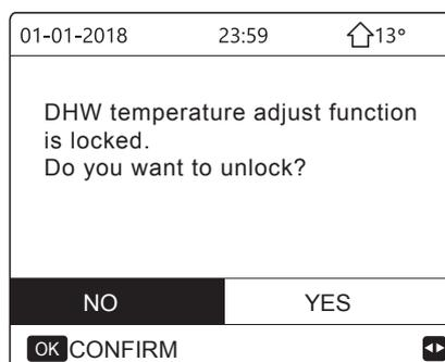
The DHW mode can't turn on or off when the DHW MODE ON/OFF is locked.If you want to turn on or off the DHW mode when DHW MODE ON/OFF is locked,the following page will appear:
