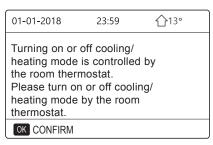
The room thermostat is SET DOUBLE ZONE(see "ROOM THERMOSTAT SETTING" in "Installation and owner's manual "). The room thermostat for fan coil is turned off, the room thermostat for the floor heating is turned on, and the unit is running, but the display is OFF. The following page is displayed:
