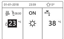
1 ) When the cursor is on the temperature of space operation mode side (Including heat mode  $\dot{\phi}$ , cool mode  $\dot{k}$  and auto mode  $\dot{A}$ ), press "ON/OFF" key to turn on/off space heating or cooling .
