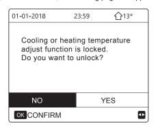
The cool/heat mode can't turn on or off when the COOL/HEAT MODE ON/OFF is locked. If you want to turn on or off the cool/heat mode when COOL/HEAT MODE ON/OFF is locked, the following page will appear:
