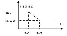
State: In the setting the wired controller, if T4C2<T4C1, then exchange their value; if T1SETC1<T1SETC2, then exchange their value.
