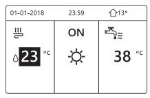
If the cursor is on the temperature, use the "◄"、 "▶" to select and use "♥"、 "▲" to adjust the temperature.
