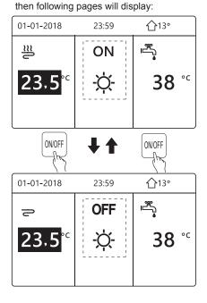
Use the room thermostat to turn on or off the unit for space heating or cooling.
