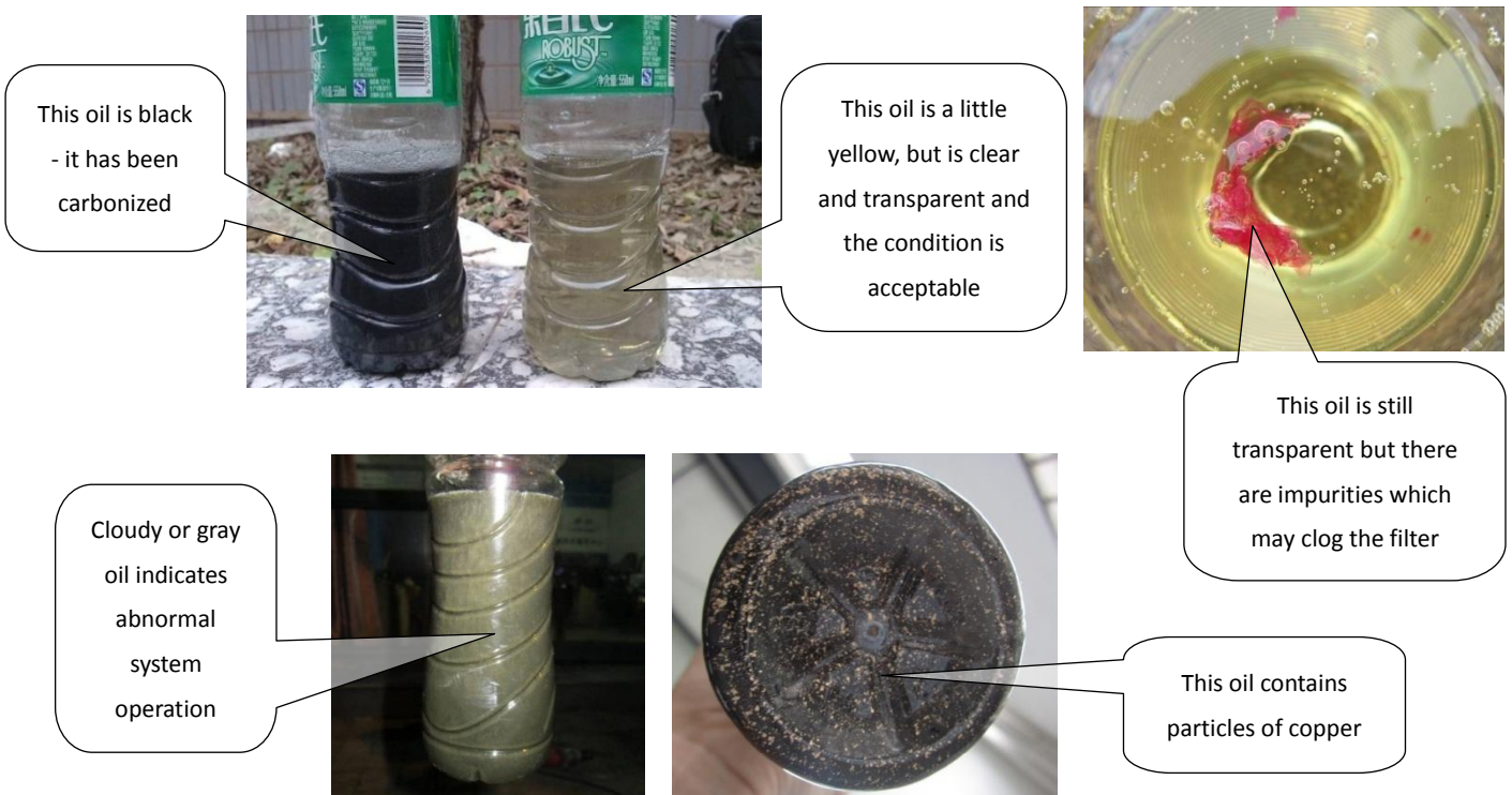
Figure 6-2.10: Inspecting compressor oil
