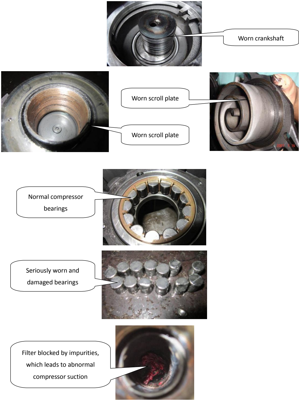
Figure 6-2.11: Effects of spoiled compressor oil
