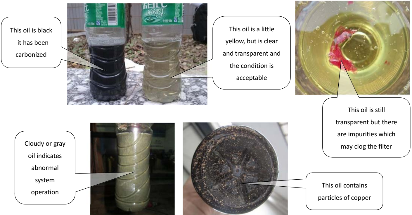
Figure 4-4.12: Inspecting compressor oil
