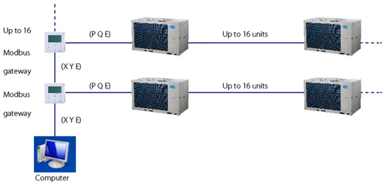
Figure 3-4.5: Modbus Gateway wiring connection
