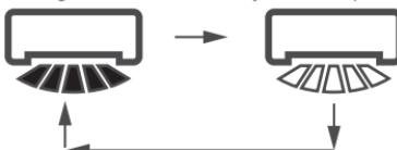
Fig.37 Horizontal louver adjustment sequence
