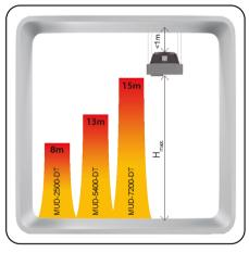
H max - Maximum height when deflectors are installed vertically
