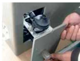
Easy maintenance. The fan and motor can be removed from the panel.
