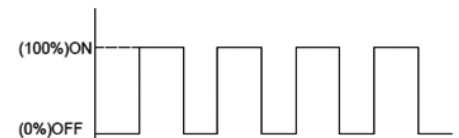
Output capacity with fixed compressor
