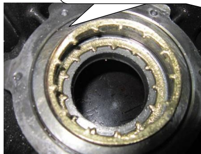
The filter is blocked by impurity, the suction of the compressor will be abnormal
