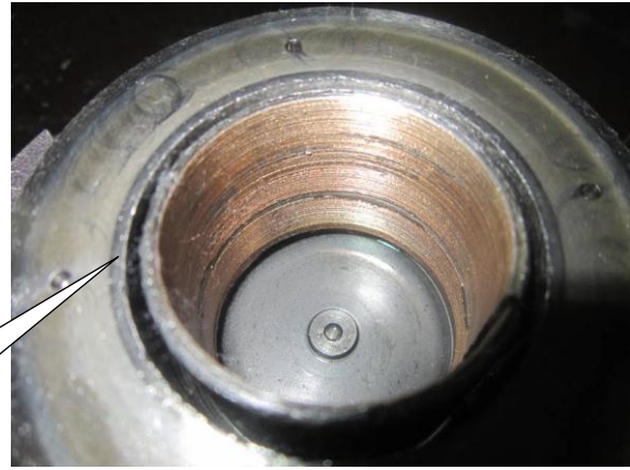
The scroll plate is worn.
