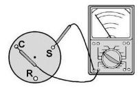
Remove compressor terminal box cover and disconnect wires from terminals. Using an ohmmeter, check continuity across the following:
