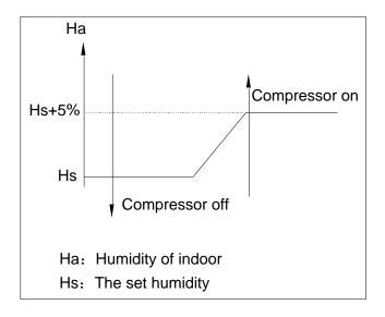
When Ha<Hs, the compressor shuts off. When Ha≥Hs+5%, the compressor will shut on according to the 3 minutes delay condition. When compressor shuts on, the fan motor operates at the same time. If it shuts off, the fan motor stops delaying for 3 minutes (except for water full and anti-freezing)
