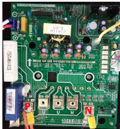
Figure 5-4.9: Inverter module terminals
