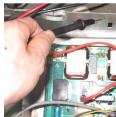
Figure 5-4.7: Measuring resistances between compressor terminals and ground
