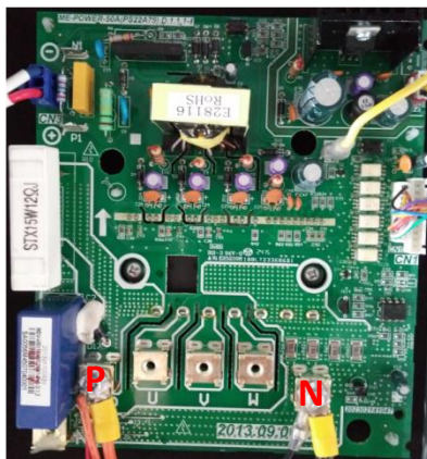
Figure 5-4.11: Inverter module terminals
