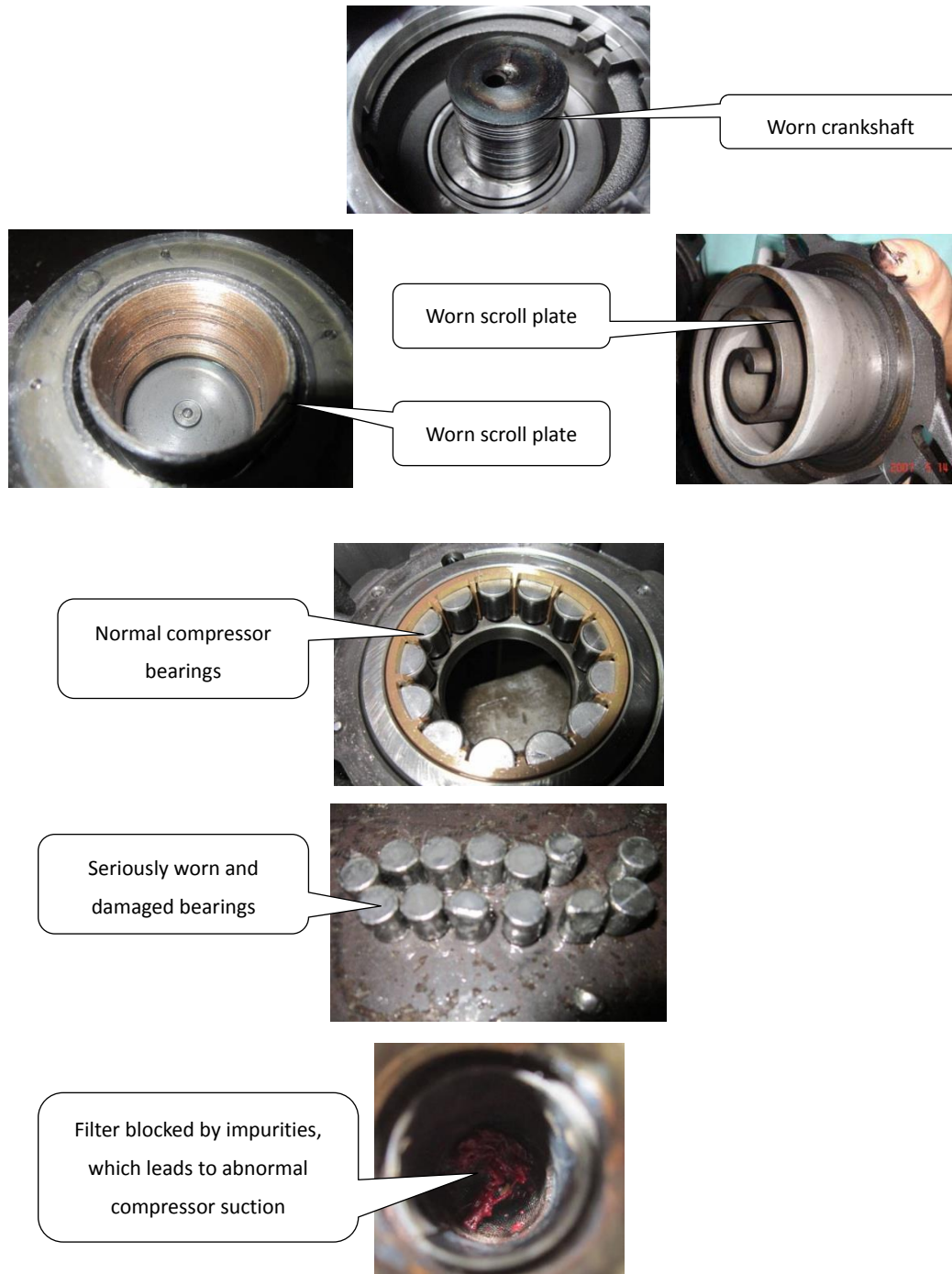
Figure 5-4.17: Effects of spoiled compressor oil
