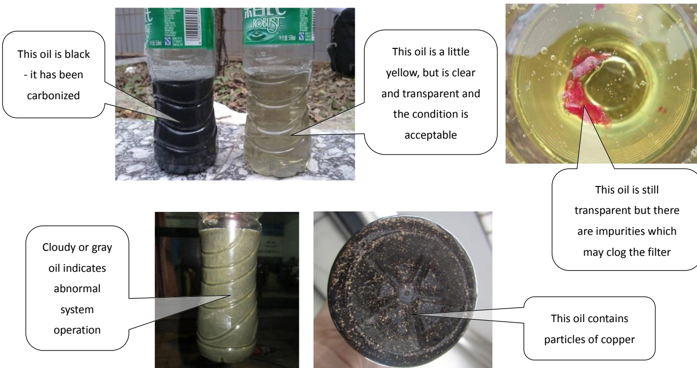
Figure 5-4.16: Inspecting compressor oil
