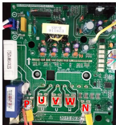
Figure 5-4.1: Inverter module terminals
