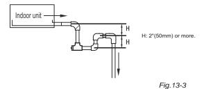
Caution: Whileconnecting the drain pipe, please use the drain pipe connect to the secondary water holder simultaneously, for avoiding there are little condensate water deposit in the unit when the machine is running under the high humidity working condition.
