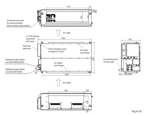
The method of installation: adopt following method if the air-conditioning's size of installation site is limited and the indoor unit can't put into the installation site.
