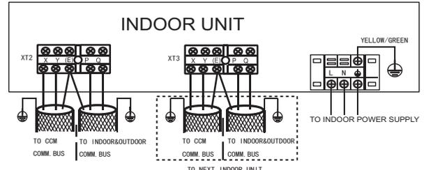
Please use 3-core shielding wire, and ground the shielding layer.
