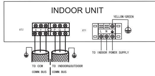
Please use 3-core shielding wire, and ground the shielding layer.
