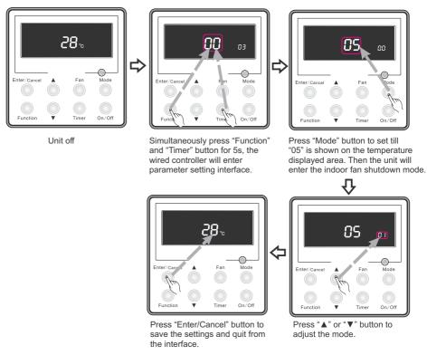
Fig.25 Indoor fan shutdown mode setting
