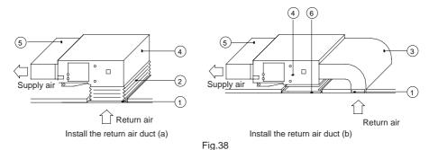
Table 10 Installation of the return air duct
