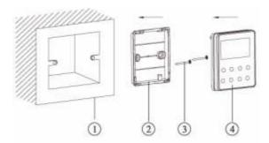
Fig.26 Standard Parts of the Wired Controller
