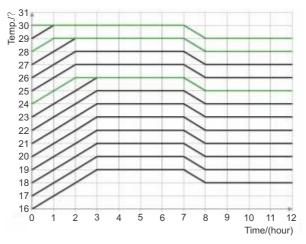
Fig.14 Sleep Curve under the COOL Mode
