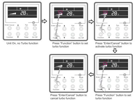
Fig.19 Turbo Function Setting
