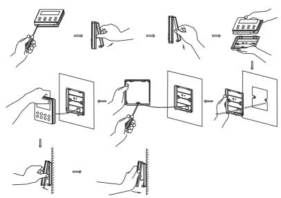
Fig.27 Installation of the Wired Controller
