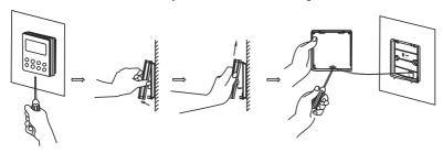
Fig.28 Removal of the Wired Controller
