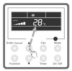
Fig.7 Temperature Setting
