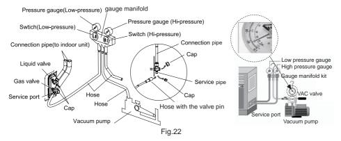
Note: For the large-sized unit, it has the service port for both the gas valve and the liquid valve. During evacuation, it is available to connect two hoses of the manifold valve assembly to two service ports to quicken the evacuating speed.
