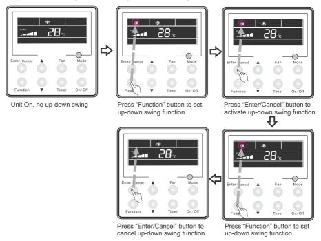
Fig.10 Up and Down Swing Setting
