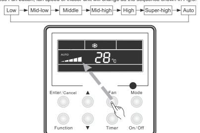
Fig.8 Fan Speed Setting
