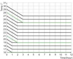
Fig.15 Sleep Curve under the HEAT Mode
