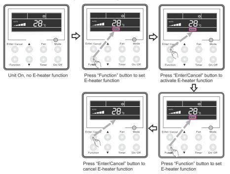
Fig.21 "E-HEATER" Function Setting
