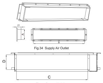
Fig.35 Return Air Inlet Table 9
