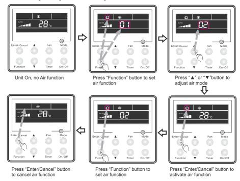
Fig.12 Air Exchange Setting
