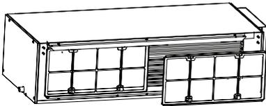
Press the return air inlet filter downward against the guide groove sponge and take it off along the arrow direction. There are two return air inlet filters.
