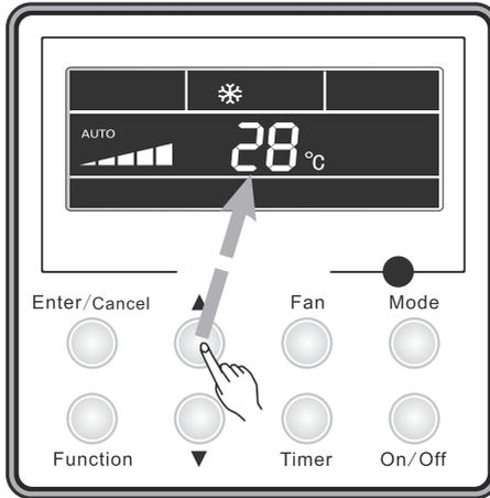
Fig.7 Temperature Setting
