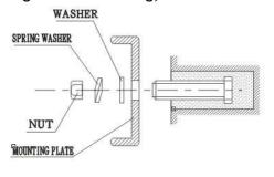
3.1.2 Fix the bolts in the proper position (Decide the position with the mounting plate and pour cement into the bolt holes.)
