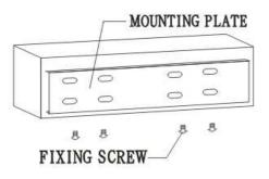
3.1.3 When the cement has freeze, fit the mounting plate (use the washer and nut according to the following)
