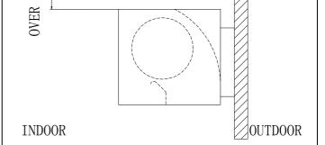
2.3 Don't install the unit too low, no less than2.3 meter from the ground.
