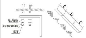
3.3.3 Set the mounting plate on the ceiling brackets and ensure safe & fixing (use the bolts attached to the ceiling brackets as Fig. Using the ceiling brackets to hang from the ceiling, the position of mounting plate can be adjusted in the limit of 100mm.
