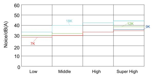
Indoor Fan Motor Rotating Speed
