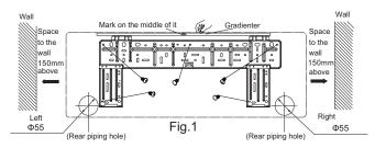
(2) Open a piping hole with the diameter of  $\Phi$ 55 or  $\Phi$ 70 on the selected outlet pipe position.In order to drain smoothly, slant the piping hole on the wall slightly downward to the outdoor side with the gradient of 5-10°.(As show in Fig.2)
