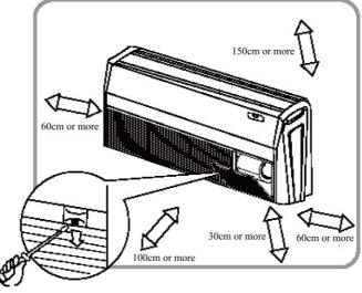
The space around the unit is adequate for ventilation. (Refer to Fig.1)
