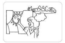
\* To distribute cool air throughout the room, adjust airflow direction as shown by the arrows (see picture) to diffuse cool air.
