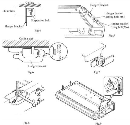
When installing the indoor unit, you can refer the paper pattern for installation, and make sure that the drainage side must be 10mm lower than the other side in order to drain the condensation water fluently.
