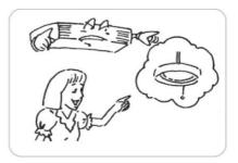
\* Do not locate any obstacle against the air flow direction of indoor and outdoor unit. Otherwise, it can cause inefficient performance or malfunction.
