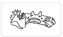
\* Do not locate a heater or any other heat source close to the unit. The heat may deform plastic parts.
