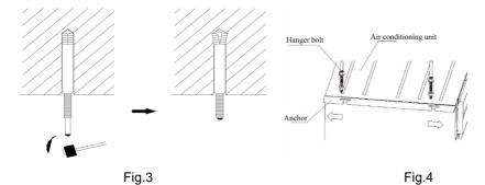
Install the hanger on the indoor unit, as shown n Fig.4.
