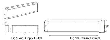
Table 4 Dimensions of the Air Supply Outlet and Return Air Inlet (unit: mm)
