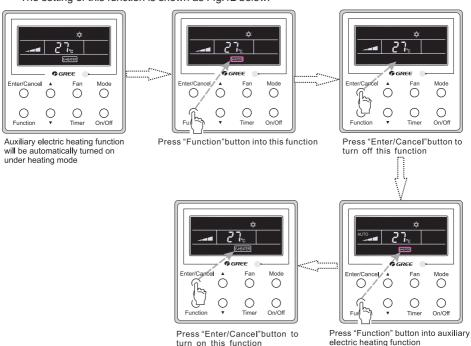
Fig.12 E-heater Setting
