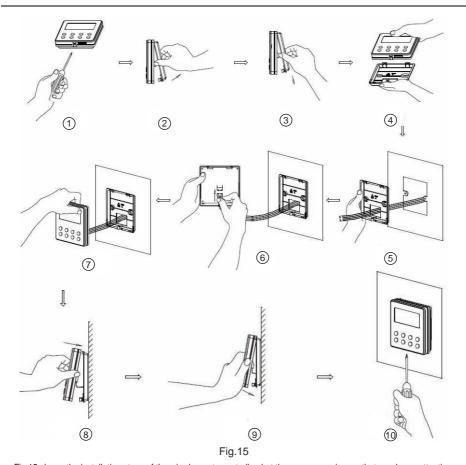
Fig.15 shows the installation steps of the wired remote controller, but there are some issues that need your attention.
