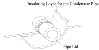
Fig.13 Thermal Insulation of the Condensate Pipe
