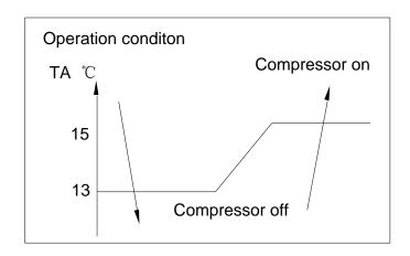
6.6.1.1 When TA<13°C, the compressor stops working. And the outdoor fan will stop delaying for 5 seconds until it operates for 3minutest.
