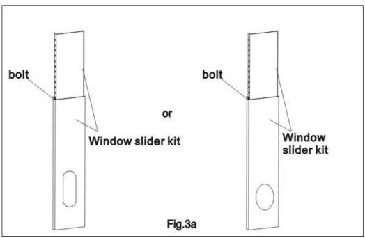
Note: If the window opening is less than the mentioned minimum length of the window slider kit, cut that one with a hole in it short to fit for the window opening. Do never cut out the hole in window slider kit.
