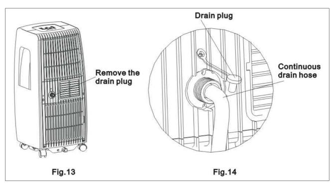
When the water level of the bottom tray reaches a predetermined level, the unit beeps 8 times, the digital display area shows "P1". At this time the air conditioning/dehumidification process will immediately stop. However, the fan motor will continue to operate (this is normal). Carefully move the unit to a drain location, remove the bottom drain plug and let the water drain away (Fig.15). Restart
