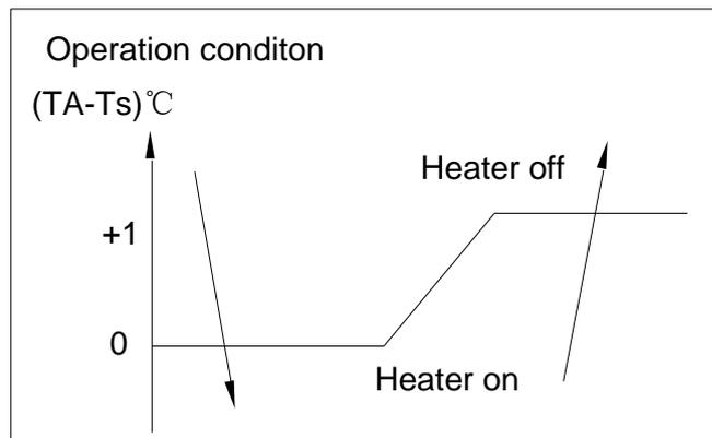
6.7.2.1. When  $TA < TS$ , the indoor fan operates firstly, and then the heater operates after 4 seconds.
