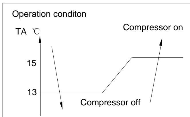
6.6.1.1 When  $TA < 13^{\circ}\text{C}$ , the compressor stops working. And the outdoor fan will stop delaying for 5 seconds until it operates for 3 minutes.
