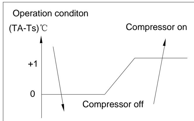
6.5.2.1 If  $TA > TS + 1^{\circ}\text{C}$ , the outdoor fan operates. After 15 seconds, the compressor operates.
