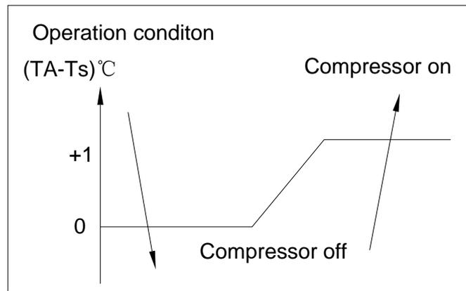
6.5.2.1 If  $TA > TS+1^{\circ}\text{C}$ , the two fans operate. After 15 seconds, the compressor operates.
