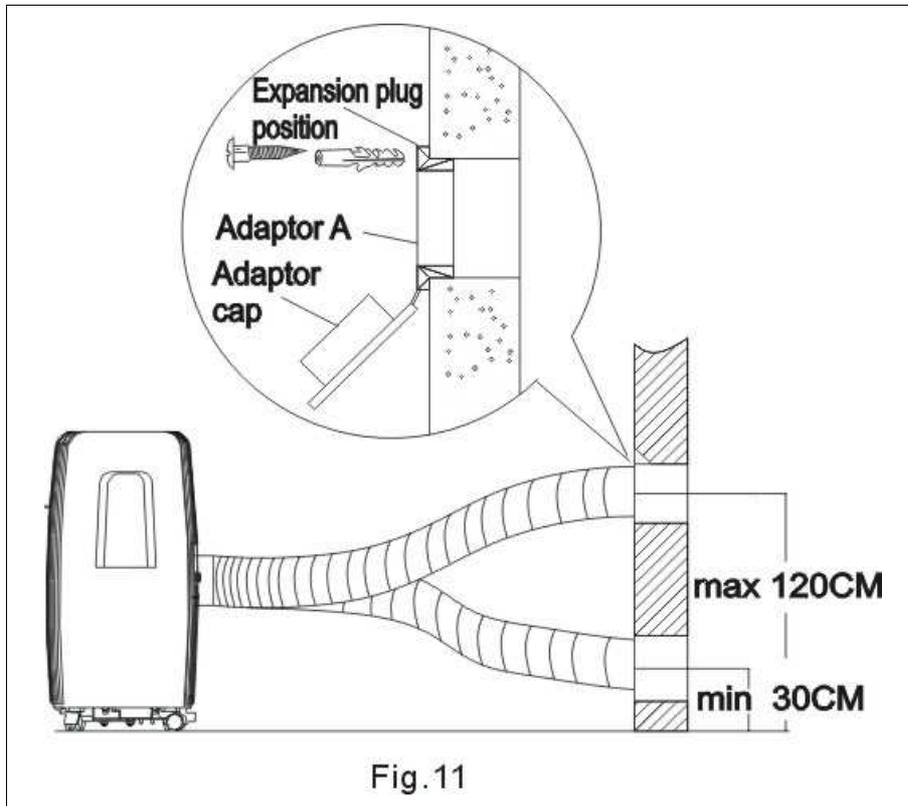
Note: Cover the hole using the adaptor cap when not in use.
