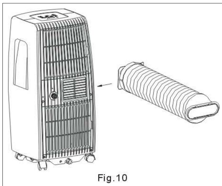
The exhaust hose can be installed into the wall!
