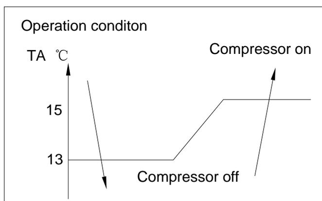
6.6.1.1 When  $TA < 13^{\circ}\text{C}$ , the compressor stops. And the two fans operate at low speed at all time.
