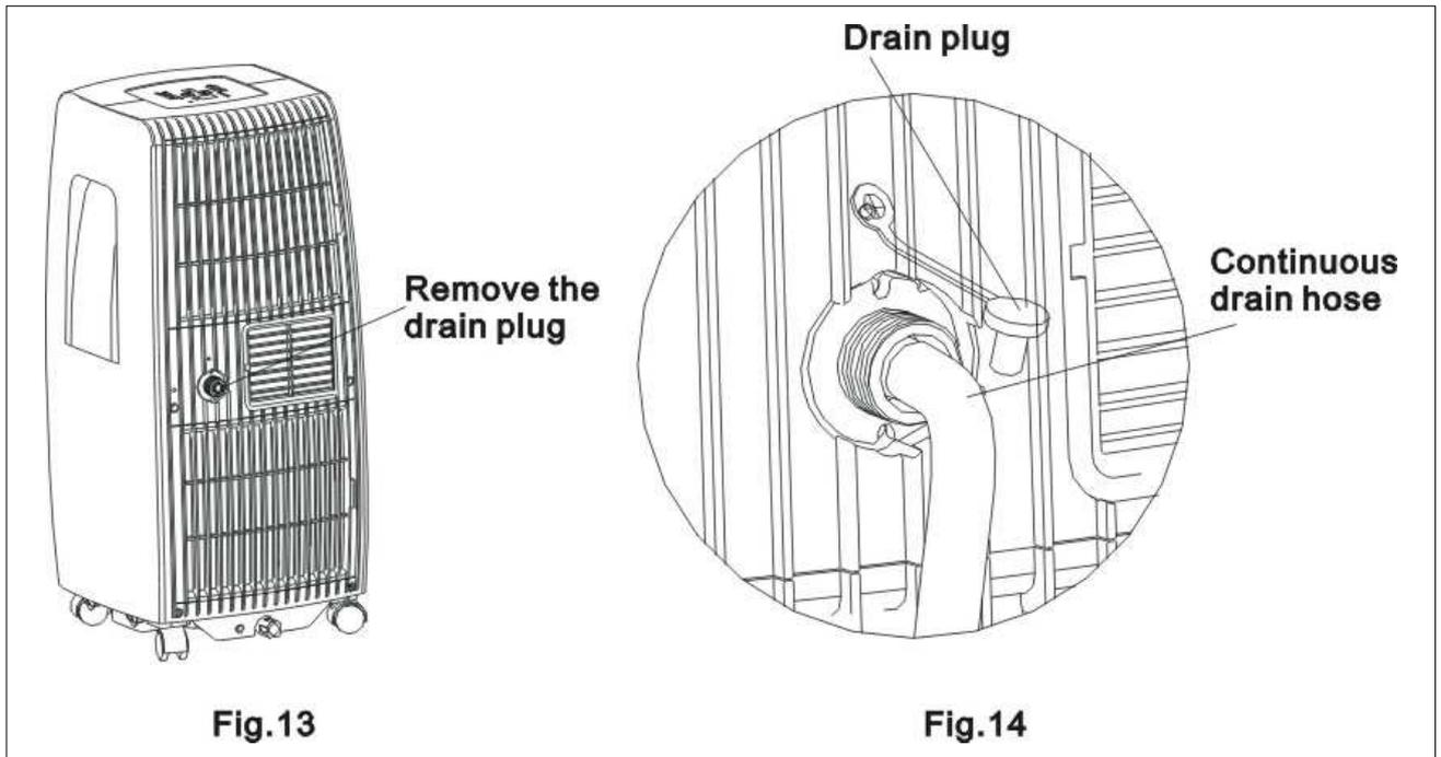
When the water level of the bottom tray reaches a predetermined level, the unit beeps 8 times, the digital display area shows "P1". At this time the air conditioning/dehumidification process will immediately stop. However, the fan motor will continue to operate (this is normal). Carefully move the unit to a drain location, remove the bottom drain plug and let the water drain away (Fig.15). Restart
