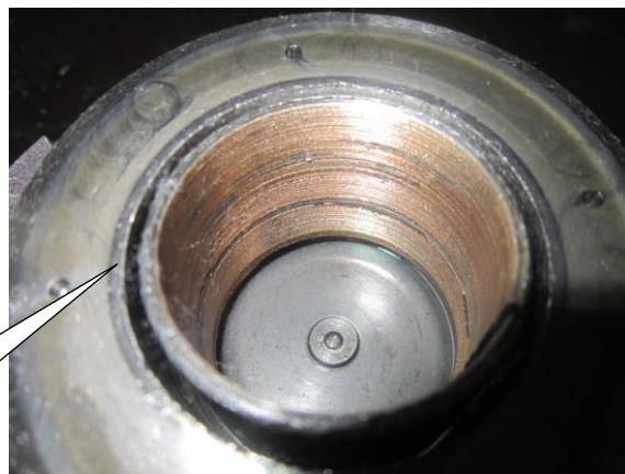
The scroll plate is worn.
