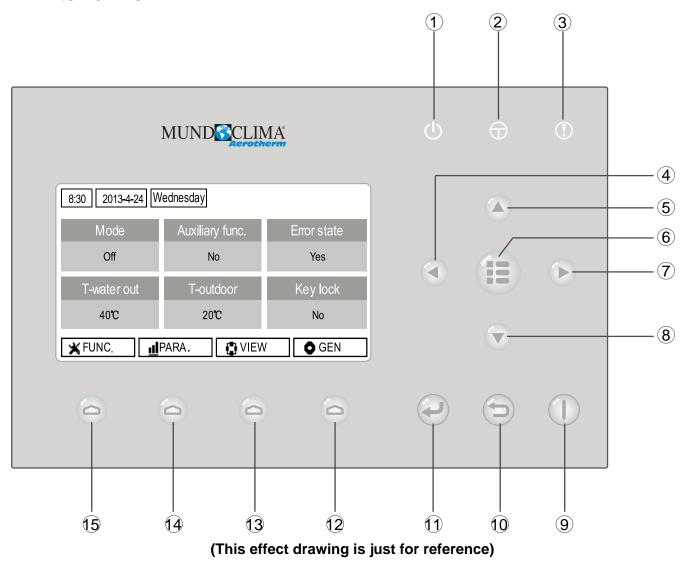
No. **Symbol** No. Symbol Description Description 1 (1) 9 Running indicating LED ON/OFF key  $\oplus$ (2) 10 Power indicating LED Cancel/Return key ① (3) 11) Error indicating LED OK key (4) (12) Left key Function key no. 4 **(5)** Up key 13 Function key no. 3 **6**) 14) Menu key Function key no. 2 (7) 15 Right key Function key no. 1 8 Down key
