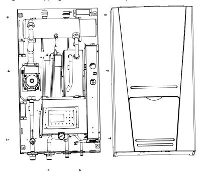
Step 2: De-installation of the control.
