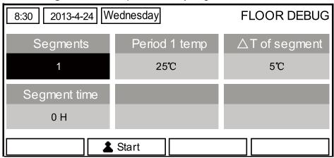
2. At the **FLOOR DEBUG** setting page, by the Left/Right key select the desired parameter and then by the Up/Down key configure it. The configurable parameters include "**Segments**", "**Period 1 temp**", "**ΔT of segment**", and "**Segment time**", as listed in the following table..
