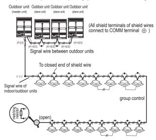
The indoor unit at the terminal of communication system should parallel connect a impedance between port P and port Q.
