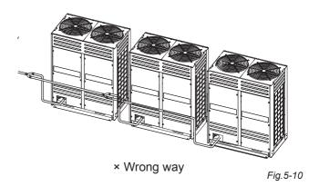
The branching pipe must be installed horizontally, error angle of it should not large than 10°. Otherwise, malfunction will be caused.
