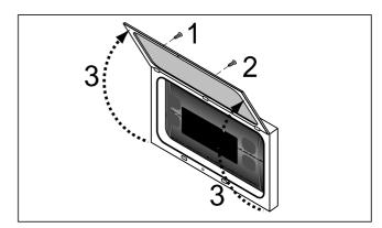
To access the control panel, open the door:
