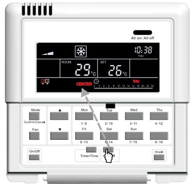
Press **“Central”** to go to the centralized control mode.
