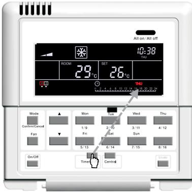
Under the single control status, press **“Timer/Time”** to go to the timing setting page.
