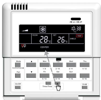
Under the single control status, press “Shield” to switch to “TEMP” .
