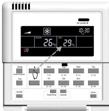
Fig.5.6 Temperature Adjustment
