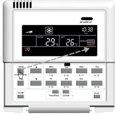
Press “Confirm/Cancel” to activate or deactivate the shielding function.
