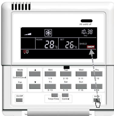
Under the single control status, press “Shield” to switch to “ ON/OFF ”.
