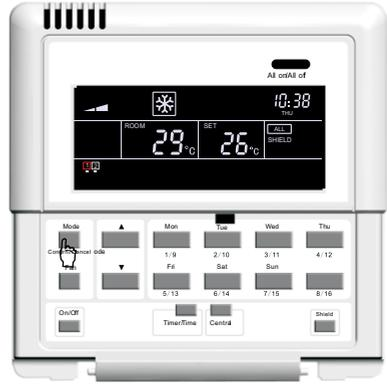
Under the single control status press “Shield” to switch to “All” .
