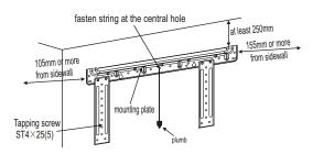
NOTICE: • The holes at solid arrow position must be secured to avoid the shake of mounting plate.
