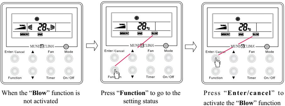
Fig. 22 How to Activate the “Blow” Function
