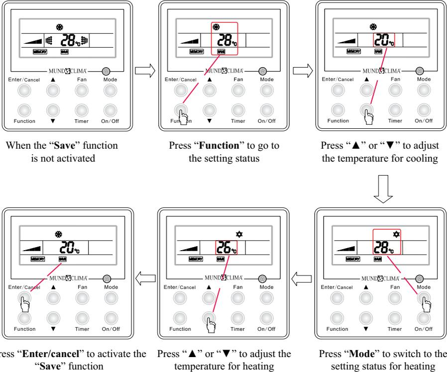
Fig. 18 How to Activate the “ Saving ” Function
