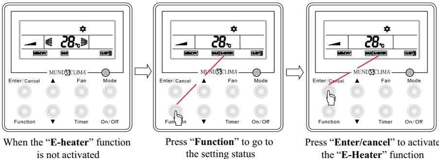
Fig. 20 How to Activate the “E-heater” function
